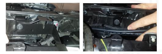
5.h. Fit the LH OTR bracket onto the mounting face for the standard radiator mounts 5.i. Place the centre OTR bracket onto the back of the bonnet latch M8 bolts 5.g. Fasten using the two nylock M8 nuts supplied in the bracket kit (M8 bolts and washers supplied if required)
