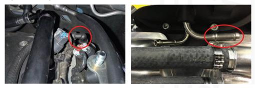
3.r. Connect the supercharger fuel hose to the hard line on the vehicle located against the firewall
