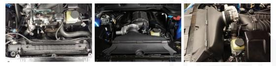
8.h. Align the grommet holes with the bosses on the radiator and gently push the OTR down until it is firmly seated on top of the radiator
