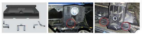
5.d. Remove the torx screw securing the washer filler bracket to the front panel.
