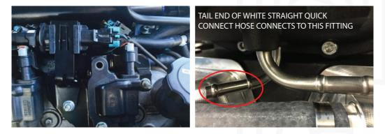
3.p. Connect the vacuum/breather from the RH head to a TEE which is connected to the valley plate vent. The other end of the TEE will connect to the OTR, see image below
