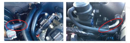
3.t. Plug the injector loom back onto the injectors ensuring that the lock clips snap down
